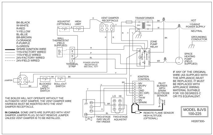
Figure 9e. Wiring Diagram, Spark Ignition, Two-Stage (BJVS 100-225).
